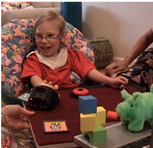
One Switch for voice-output "Build up the blocks!" and the second switch to control the battery-operated pig that knocks them down.
